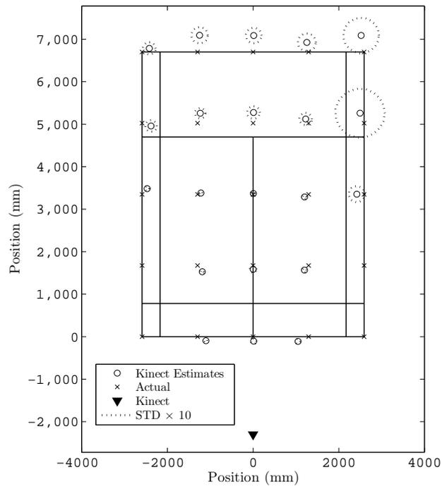
Figure 1: Positions of the participant estimated by the Kinect-based system at each of the predetermined reference grid positions on the badminton court. The standard deviation of prediction ( $\times 10$ ) is shown to illustrate the variation in prediction according to court position
