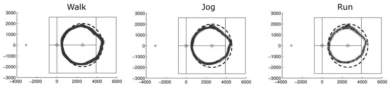
Figure 2: Circular trajectories measured using the Kinect with the participant moving at different speeds. The cross hairs indicate the trajectory of the player over three laps. The dotted line indicates the reference trajectory. The cross indicates the location of the Kinect
